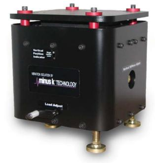
Low frequency vibration isolator for weight loads from 50 to 800 lbs. and 1/2 Hz performance vertical and horizontal.
